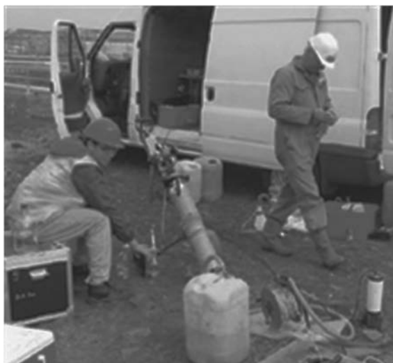
Figure 8.2. Sampling of groundwater for determination of hydrocarbon contamination
