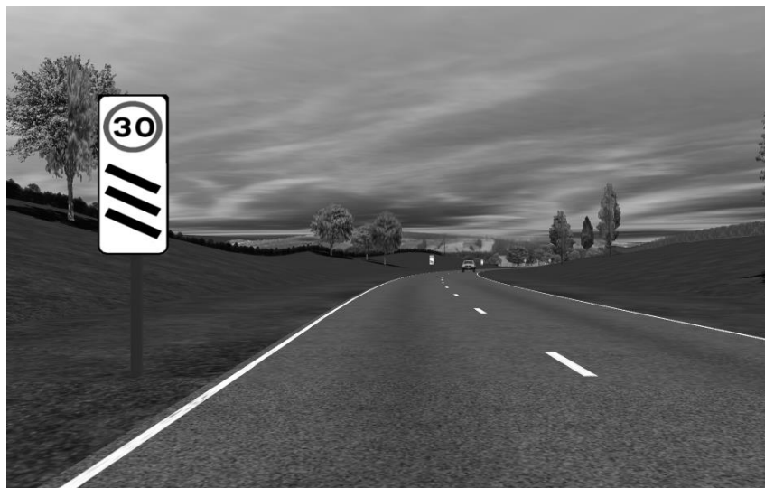
Figure 6.7. Recommended treatment for approach to village
