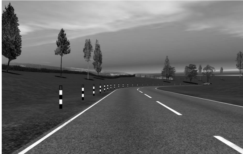
Figure 6.6. Recommended treatment for approach to rural bend
